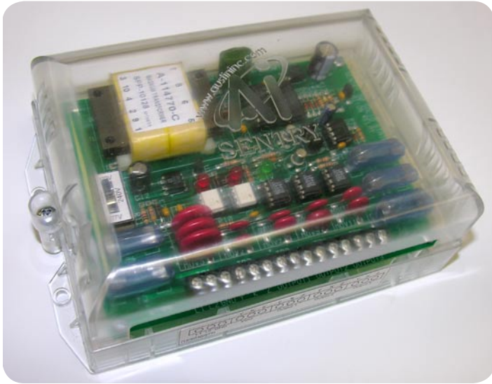
Sentry 50 unit without optional enclosure is furnished with a clear polycarbonate cover
